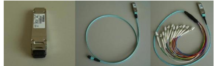
QSFP-40G-SR4 with direct MPO and 4x10 MPO-to-LC duplex splitter fibre cables
