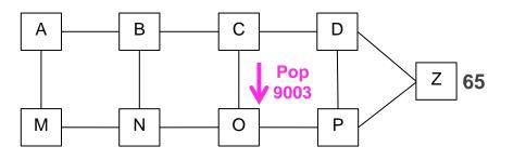
A packet injected at node C with label 9003 is forced through datalink CO
