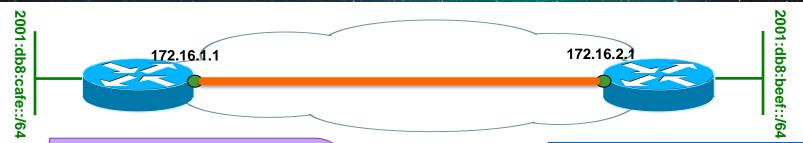
nterface Tunnel0 ipv6 address FE80::1 link-local ipv6 osof 1 area 0
