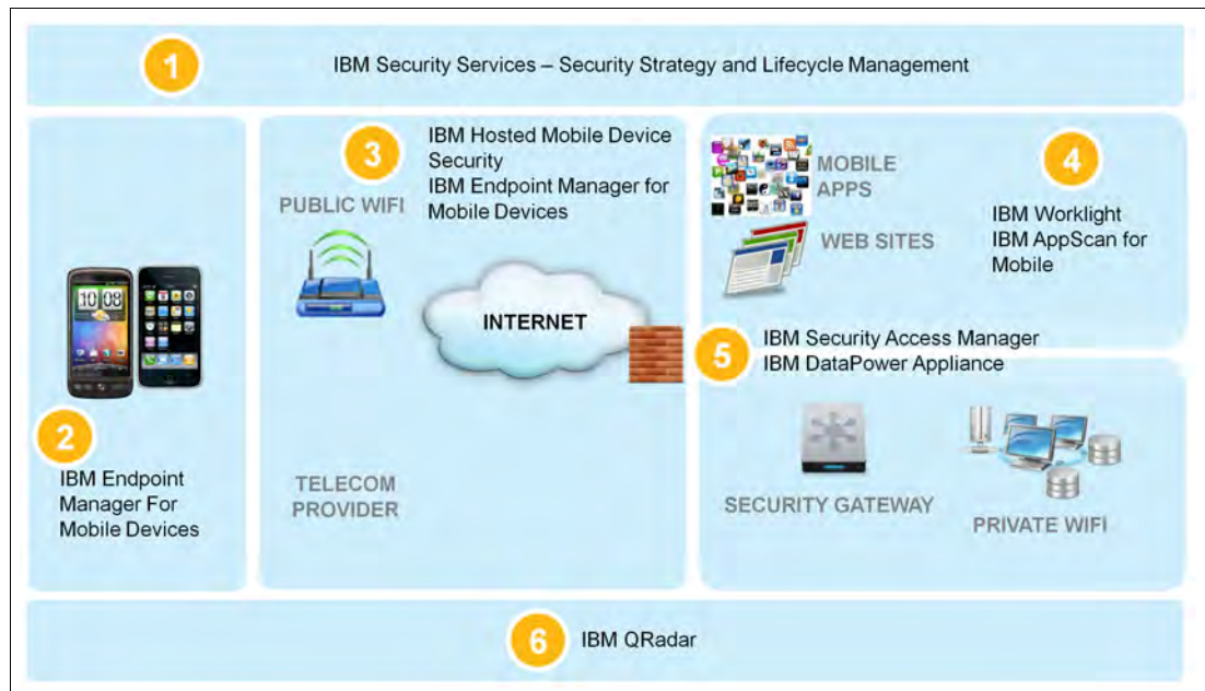
Figure 28 IBM mobile security solution deployment
